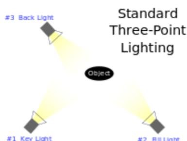
A typical three-point lighting setup
